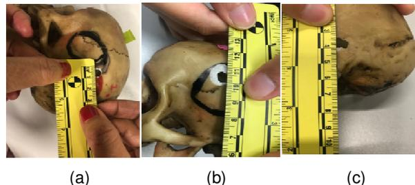
**Fig. 3.** Pattern injuries of three different artificial skulls fired at temporal position with 0.22 caliber at 10 m firing range. Fig. 3 (a), (b) (c) showed respectively the measurements taken for the entrance wound allowing the calculation of the projectile impact ratio for each skull.
