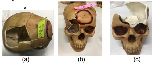
**Fig. 4.** The fracture pattern of three different artificial skulls fired at frontal position with 0.38-caliber. Fig. 4 (a), (b), (c) shows respectively the fracture injury for each skull.
