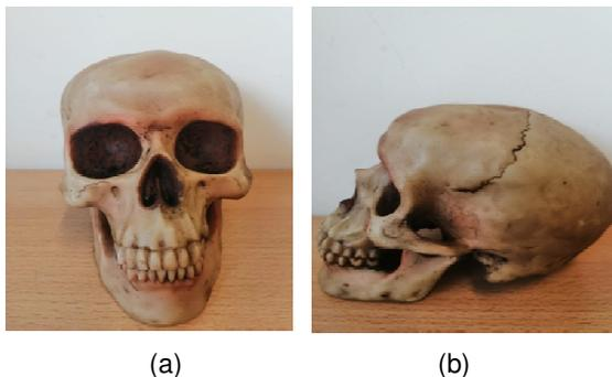
**Fig. 1.** Artificial skulls used for forensic ballistic experiments. Two different positions of firing were chosen for the experiments: (a) Frontal position, (b) Temporal position.
